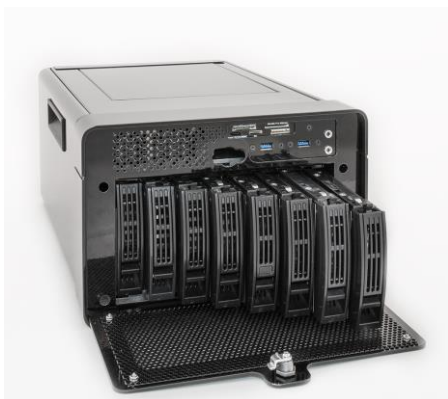
LTNG-XD-8-MMDT door open, view of disk canisters. LTNG-XD-8-MM2U inside view, cover removed.
